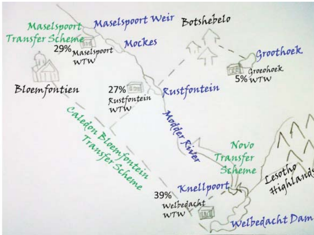
Figure 39: Schematic for the Greater Bloemfontein WSS showing the three transfer schemes in green and the percentage each Water Treatment Works supplies. All the water originates from the Caledon River with transfers into the Modder River.
