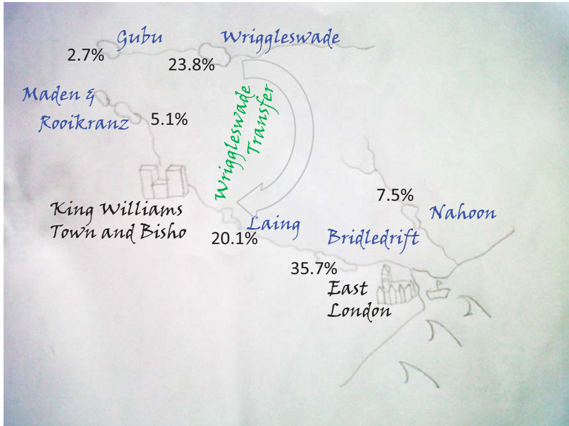
Figure 41: Benefit shed for the Amatole WSS showing the main dams which supply the scheme and the Wriggleswade transfer scheme. The percentages represent the various yields of the dams and include the transfer losses from Wriggleswade Dam.
