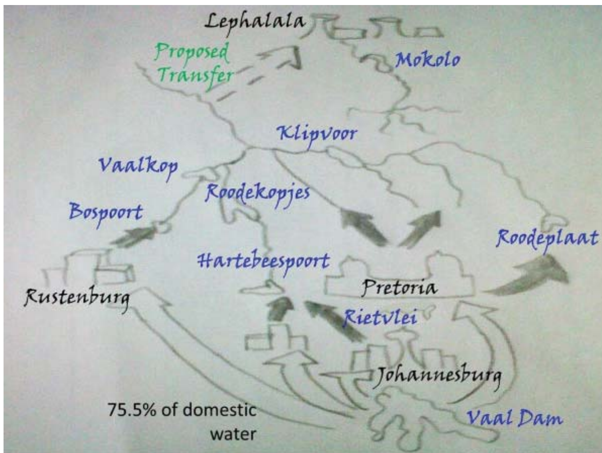
Figure 37: Schematic showing the interbasin transfers into the Crocodile West Catchment from the Vaal River System. This accounts for 75.5% of domestic water use, and 48.6% of total water use. The return flows are shown in shaded arrows. Return flows account for 29% of the water balance for the catchment.
